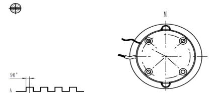
Rated Voltage 24 VDC Rated Power 130W Rated Torque 0.62 Nm Rated Speed 2000 Rpm **Duty Cycle** S2 (5 Mins) IP54 Protection Magnetic Encoder 12 PPR **Brake Holding Torque** 1.5Nm min. Brake Voltage 24 VDC Brake Pull-In Voltage 3.5 to 6V Brake Release Voltage <3V
